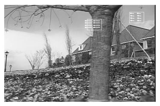
Fig. 3.3 Smoothness Constraint: Constant motion is assumed for a small neighborhood
