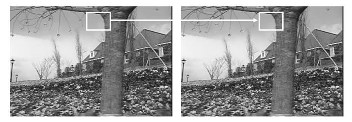
Fig. 3.1 Data Conservation: Although it has moved, the highlighted region on the right looks roughly the same with the region on the left.
